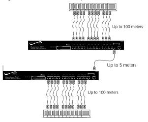
Cascade up to six StackMaster TX12 hub, using SCSI cascade connectors at the back, to provide seventy-two RJ-45 Fast Ethernet port connections.
